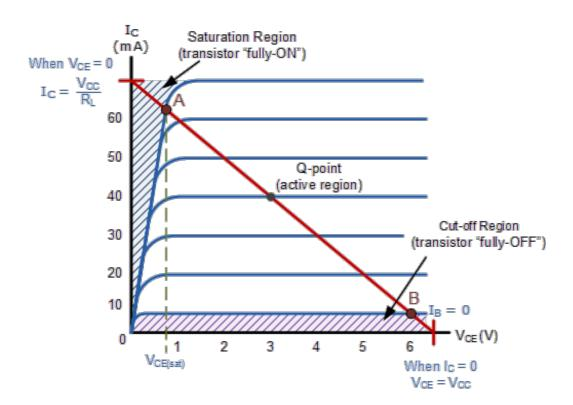
The pink shaded area at the bottom of the curves represents the "Cut-off" region while the blue area to the left represents the "Saturation" region of the transistor. Both these transistor regions are defined as:
