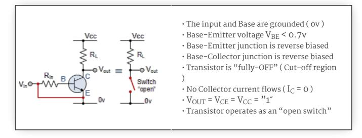
Then we can define the "cut-off region" or "OFF mode" when using a bipolar transistor as a switch as being, both junctions reverse biased, V<sub>B</sub> < 0.7v and I<sub>C</sub> = 0. For a PNP transistor, the Emitter potential must be negative with respect to the Base.
