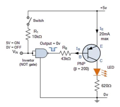
The equations for calculating the Base resistance, Collector current and voltages are exactly the same as for the previous NPN transistor switch. The difference this time is that we are switching power with a PNP transistor (sourcing current) instead of switching ground with an NPN transistor (sinking current).
