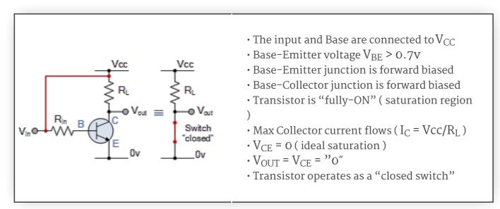
Then we can define the "saturation region" or "ON mode" when using a bipolar transistor as a switch as being, both junctions forward biased, V<sub>B</sub> > 0.7v and I<sub>C</sub> = Maximum. For a PNP transistor, the Emitter potential must be positive with respect to the Base.
