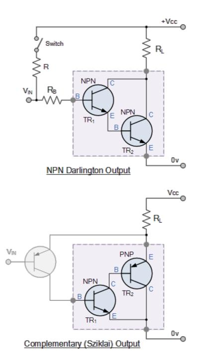
The above NPN Darlington transistor switch configuration shows the Collectors of the two transistors connected together with the Emitter of the first transistor connected to the Base terminal of the second transistor therefore, the Emitter current of the first transistor becomes the Base current of the second transistor switching it "ON".
