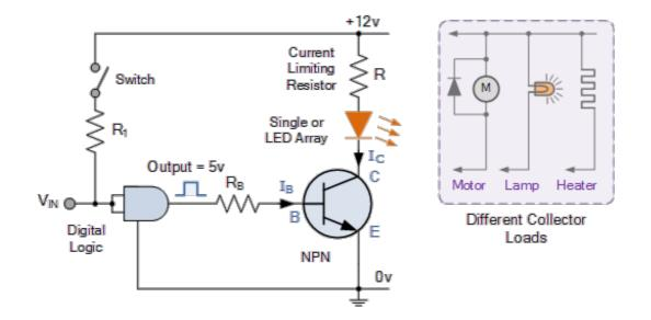
The base resistor, Rb is required to limit the output current from the logic gate.
