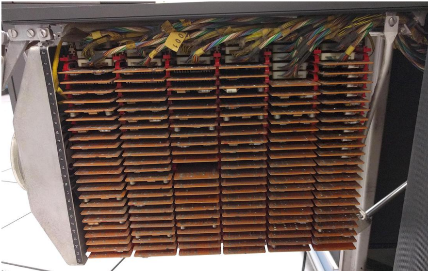
SMS cards installed in the IBM 1401 computer. The fan at the left keeps the cards cool.
